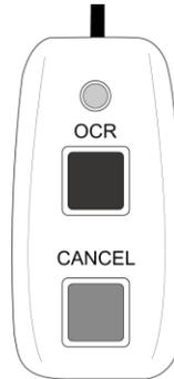
Hold the remote in your hand so that the end with the micro USB port is facing you. The remote contains 2 buttons. The top most button is the "OCR" button, and the bottom most button is the "Cancel" button. These buttons have the same functions as the equivalent buttons on the Blaze EZ.
